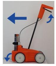
11- Swing the marking target into position, line-up on the chalk line or the existing line, press on the trigger and start your marking. Your pace should be at 30 seconds for 10 meters.
