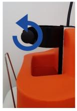
7- Unscrew the aerosol collar holder to ease the insertion of the paint can.
