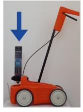
8- Insert the Tracing PRO can vertically until the Soppec PureSPRAY™ nozzle is positionned into the spray activation module.
