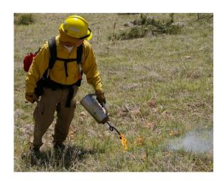
Drip torch used in direct attack to generate controlled fire lines in a comfortable and safe way. Made of aluminium, available in two models:
